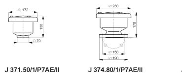
■ J 34x - deflagration flame arresters - end-of-line with overpressure and underpressure valves
