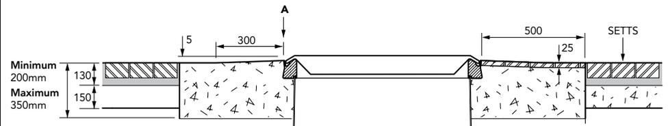
766mm x 766mm raised composite cover with an aluminium frame.
