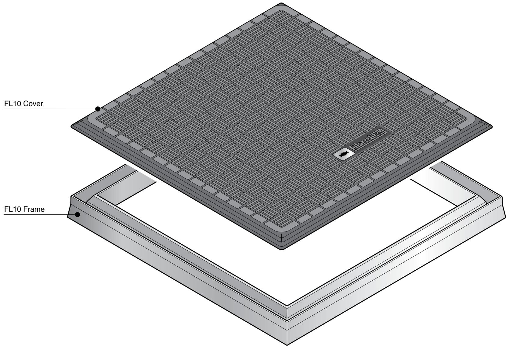
766mm x 766mm raised composite cover with an aluminium frame.
