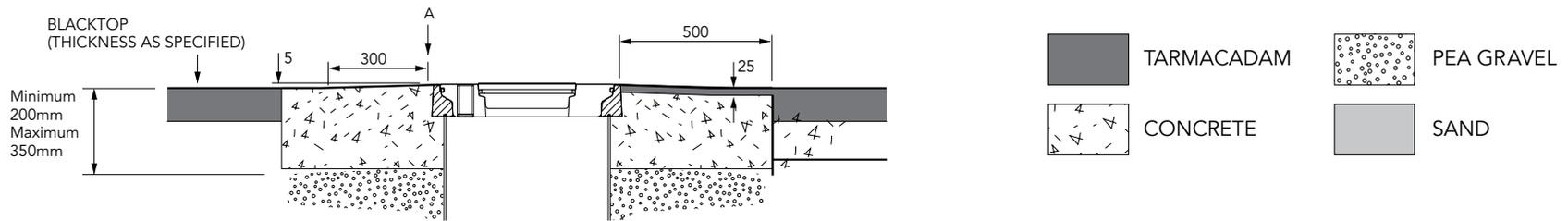
457mm diameter flat sealed composite cover and frame with a central fill port cover.
