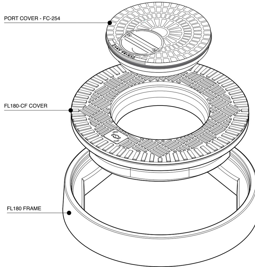
457mm diameter flat sealed composite cover and frame with a central fill port cover.
