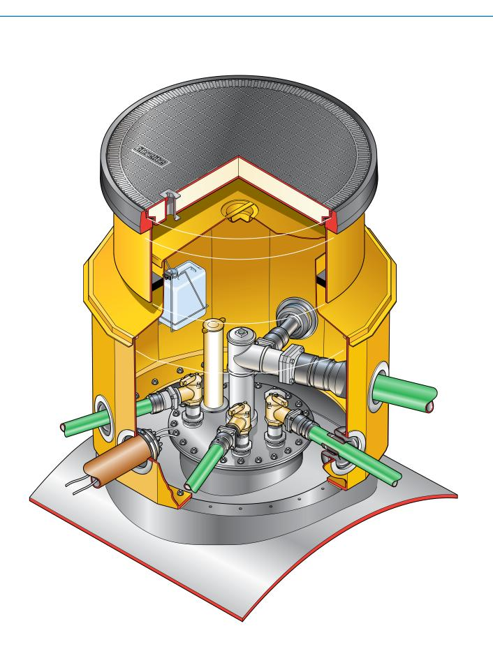
1.2m diameter bolted base chamber, corbel, internal lid with a height adjustable skirt and round 900mm flat sealed cover. Sealkit with condensation bottle and fixing kit. Round tank flange. Remote Fill
