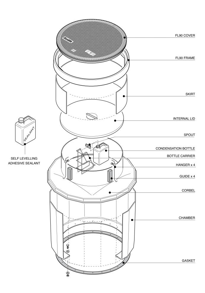
1.2m diameter bolted base chamber, corbel, internal lid with a height adjustable skirt and round 900mm flat sealed cover. Sealkit with condensation bottle and fixing kit. Round tank flange. Remote Fill
