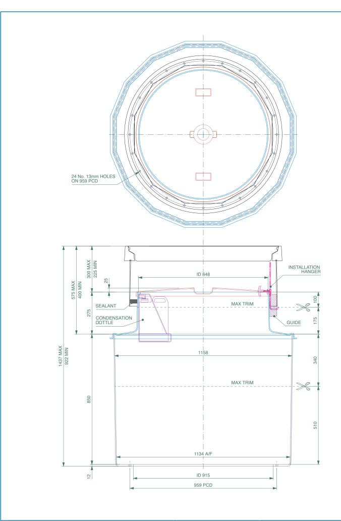
1.2m diameter bolted base chamber, corbel, internal lid with a height adjustable skirt and round 900mm flat sealed cover. Sealkit with condensation bottle and fixing kit. Round tank flange. Remote Fill
