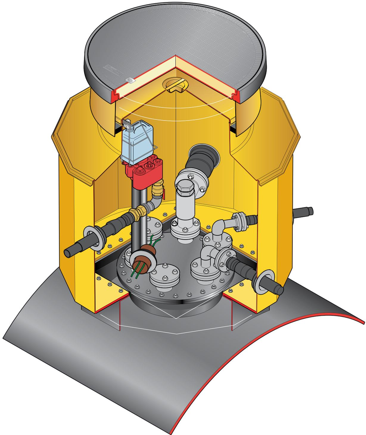
1.5m diameter 12 sided sump with solid base and manway lid adaptor, corbel, adjustable height skirt, internal lid, and round 1020mm flat sealed cover and frame
