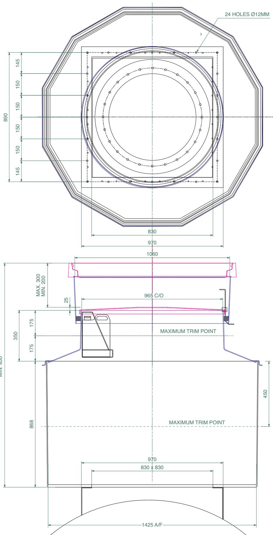
1.5m diameter 12 sided sump with solid base and manway lid adaptor, corbel, adjustable height skirt, internal lid, and round 1020mm flat sealed cover and frame
