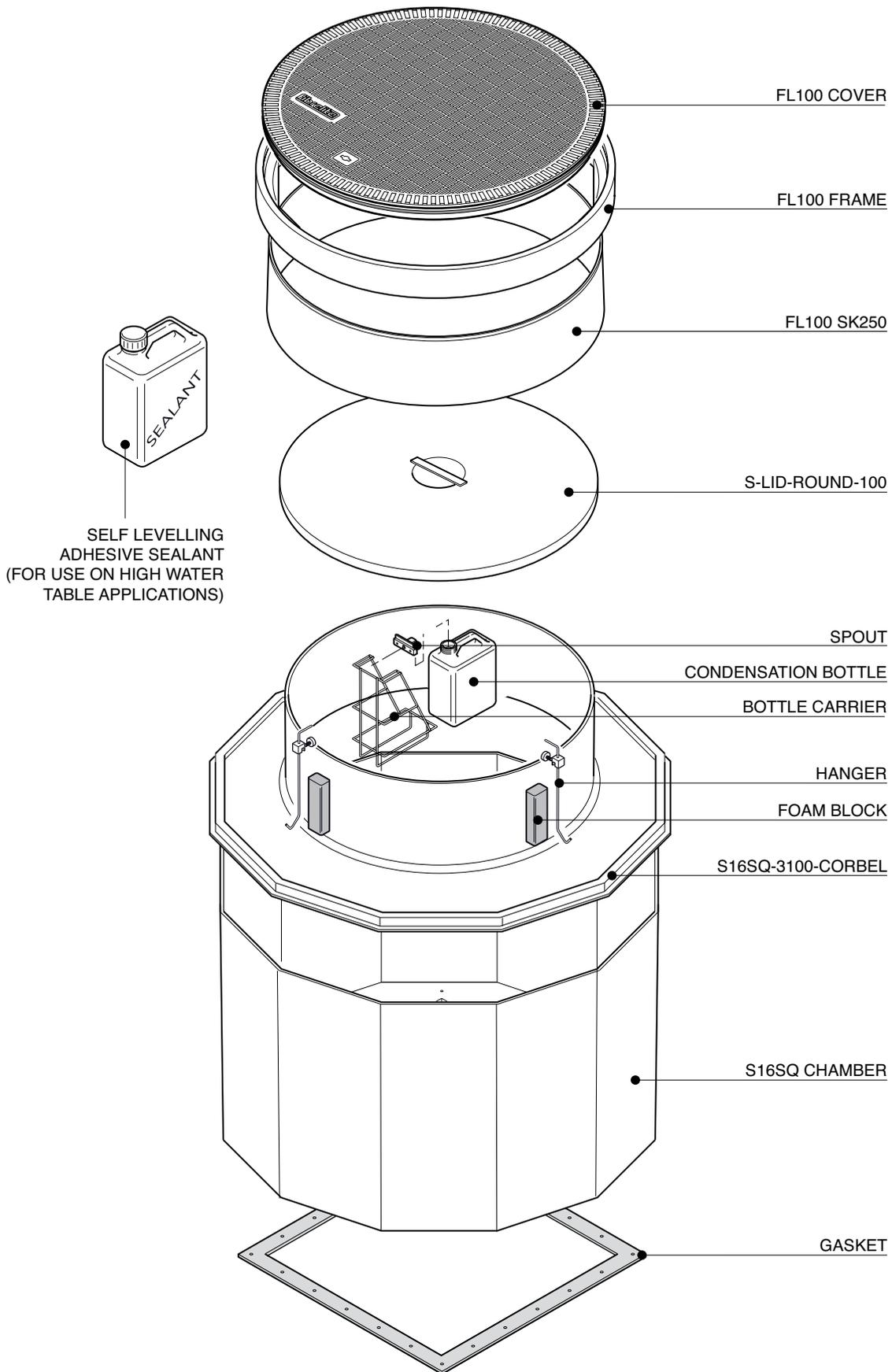
1.5m diameter 12 sided sump with solid base and manway lid adaptor, corbel, adjustable height skirt, internal lid, and round 1020mm flat sealed cover and frame
