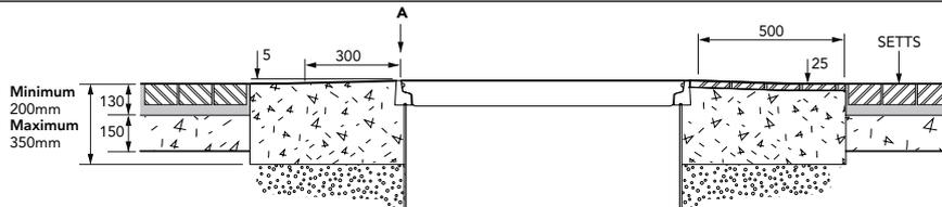
1.5m diameter 12 sided sump with solid base and manway lid adaptor, corbel, adjustable height skirt, internal lid, and round 1020mm flat sealed cover and frame
