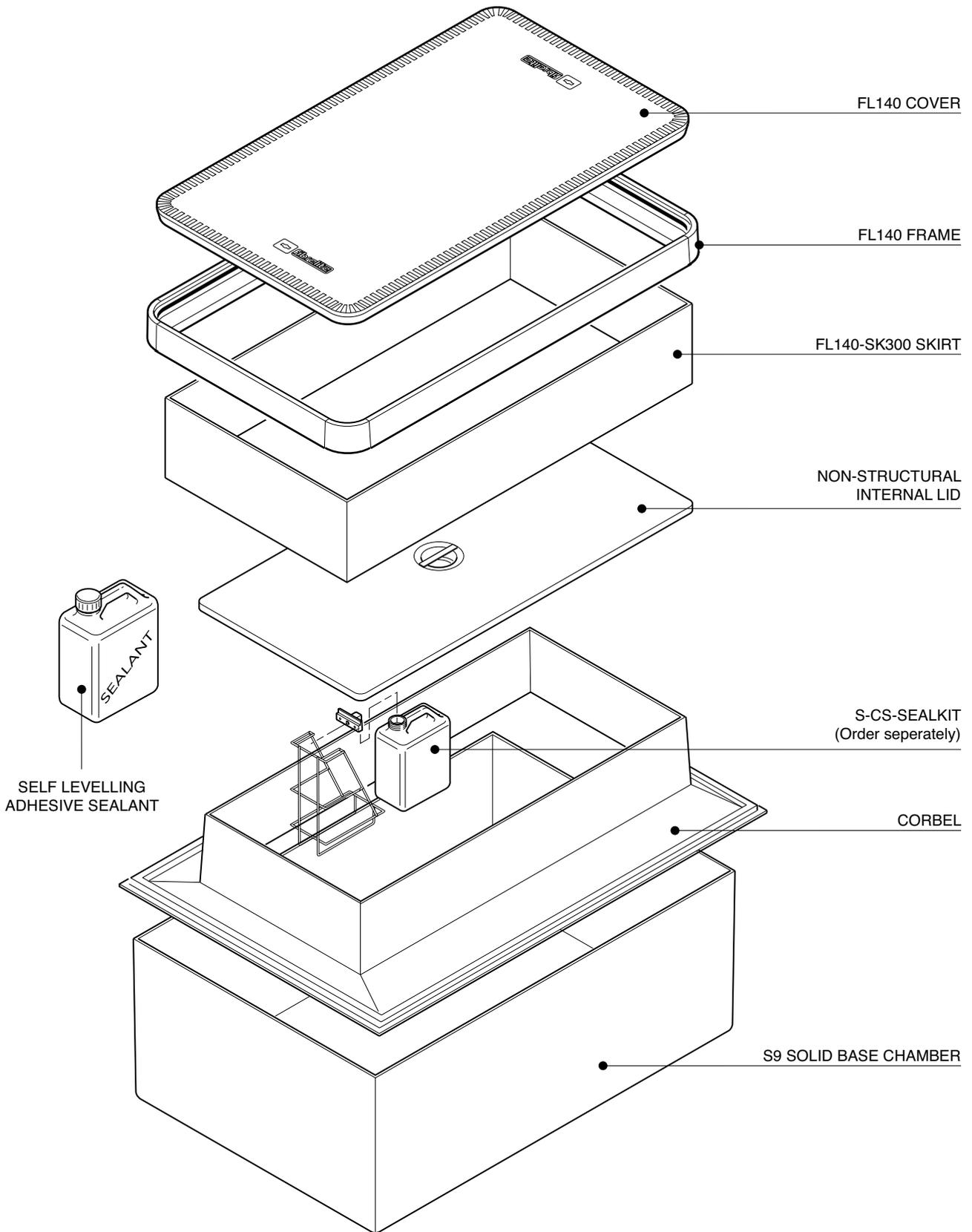
1470 x 990mm solid base chamber, corbel, adjustable skirt, internal lid and flat sealed cover with frame.
