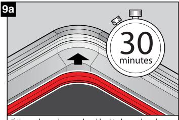
If the seal was damaged and had to be replaced allow the glue to cure (approx 30 mins) and refer to the Seal Replacement Instructions (pages 2-3, steps 1-11), if not proceed.
