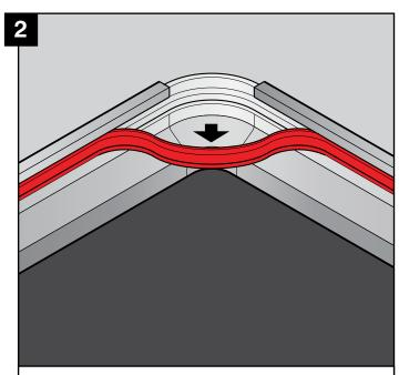
Pull the seal out to ensure it does not get damaged or trapped in the process of replacing the corner casting.
