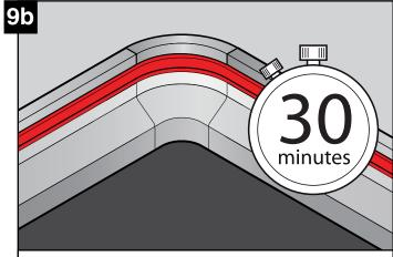
When the glue is cured (approx 30 mins) fit the seal back into the retaining recess
