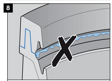
Remove any excess glue from the recess that carries the seal. Failure to do this may result in the seal not "seating" correctly
