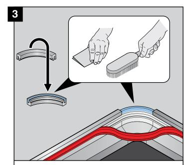
Thoroughly abrade the adhesive contact areas of the corner castings (DO NOT USE SOLVENTS) to remove any debris or glue residue. This can be achieved by using a wire brush or sandpaper. Remove any dust with a clean dry cloth.
