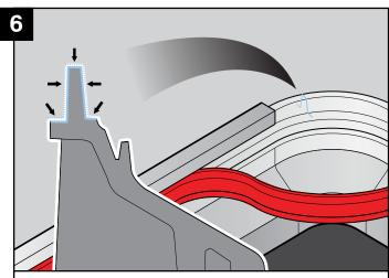
After mixing immediately apply the adhesive to the horizontal joint face and vertical tangs of the base casting.
