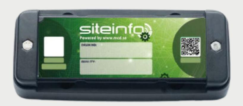
Together with our cloud service Sitelnfo, you are able to plan efficient logistics, and avoid empty drums. The standalone sensor uses ToF (Time of Flight) to detect product levels. The sensor reports the levels every 8th hour. If the consumption exceeds 10 liters during 1 hour, the frequency of reports increases during the time that the consumption is elevated.
